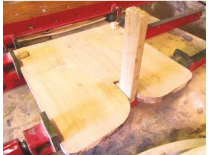
▲ Pic. 3 The seat-base was cut from front to back to accommodate a post swivelling on a dowel. The cut followed dark grain markings to hide the glue-line
